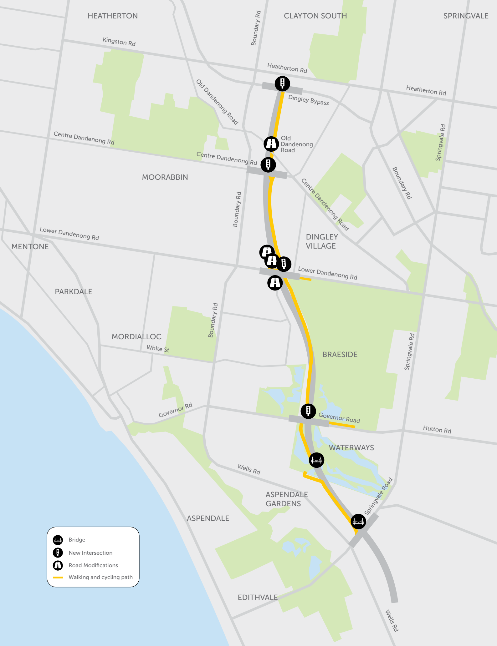
MORDIALLOC BYPASS CONCEPT DESIGN: 9 kilometers of new road, 2 new bridges, 4 new intersections and a cycle and pedestrian path along the full length of the Bypass
